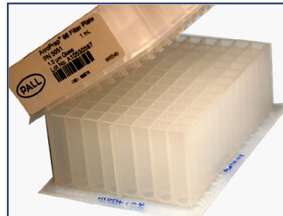
Bind & wash on a square-well block.
